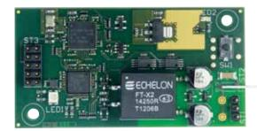
The Easylon USB Socket Interface meets the requirements of device manufacturers for an integrated LonWorks interface. Connected to the motherboard by USB the plug-in module with FTX transceiver realizes the connection to the LonWorks network. Additionally OEM variants can be realized with EIA-485 transceiver.
