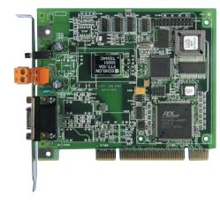
The Easylon PCI-Bus Interface is a LonTalk adapter connecting PCI-bus PCs to LonWorks and other EIA-709.1 compatible control networks.
