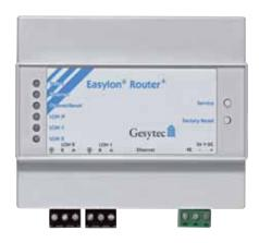
The Easylon Router<sup>+</sup> connects ISO/IEC 14908-2 compatible network segments, as well as TP/FT-10 and LON/IP-852 networks, according to the ISO/IEC 14908-4 standard. Furthermore the device operates as configuration server in LON/IP networks.
