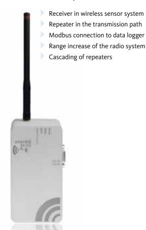
Receiver and Repeater of the GESYSENSE® wireless sensor network are devices identical in construction but for different use, which is set at commissioning. They are reception and emitting devices operating within the 433 MHz (Europe) or 915 MHz (America) ISM band
