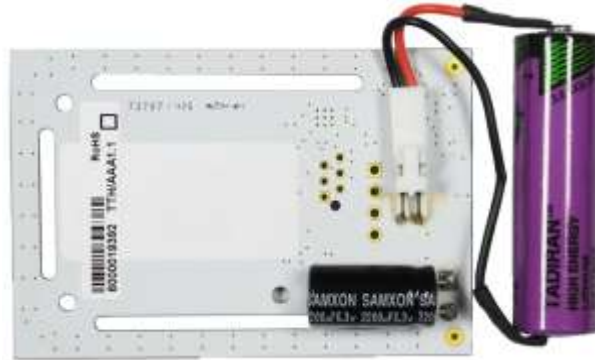
Fitting position of the battery and cable run
