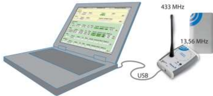
Figure 11-2: GesySense Configurator, radio adapter between PC and wireless modules
