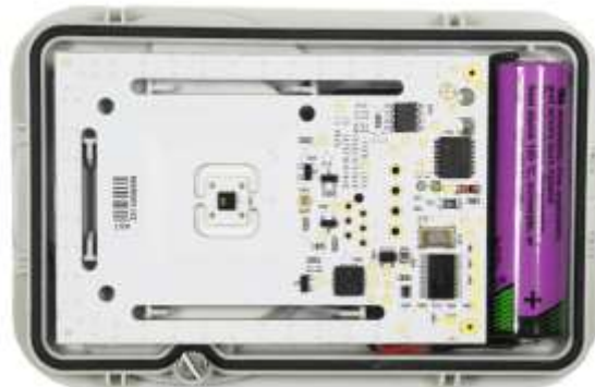
Position of board and battery inside the sensor housing
