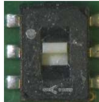
DIP switch in operating mode
